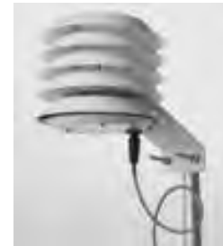
temperature probe, barometer, and radiation shield combined
